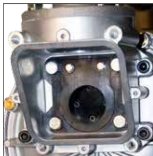
Only 4 bolts to access flap valves
